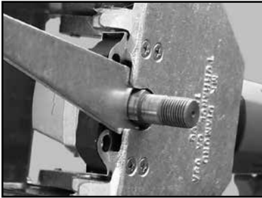
(D) Place the Shaft Wrench between the Inner Blade Guard and the Motor and onto the Motor Shaft
