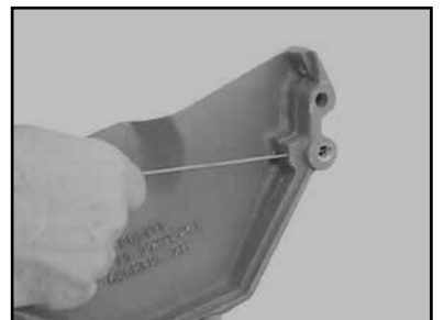
(I) Rod Cooling Channels and recheck flow
