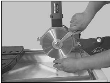
(G) Install the Retaining Nut and Outer Flange and then tighten using the Blade and Shaft Wrenches
