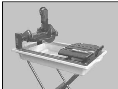
(B) Inspect Tile Saw for damage
