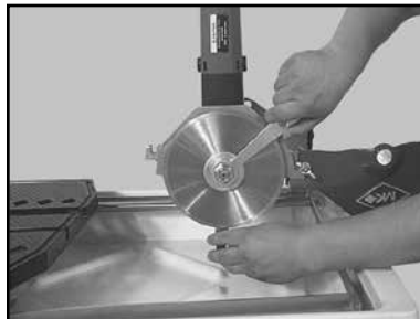
(E) Install the Retaining Nut and Outer Flange and then tighten using the Blade and Shaft Wrenches
