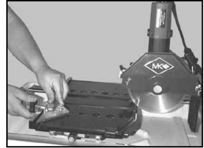
(C) Position the Dual 45° Flat Angle Guide and tighten the retaining knob
