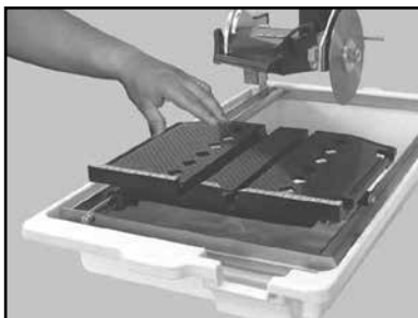
(D) Move Guide Bar and table until Square rests evenly across Blade
