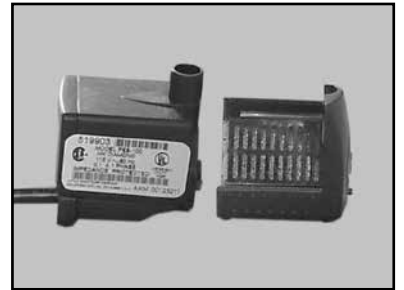
(F) Remove the Pump Intake Screen and check for debris
