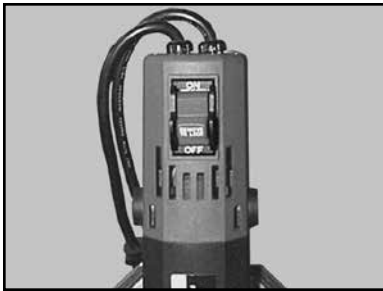
(D) Ensure the ON/OFF Switch is in the OFF position. Unplug the saw from the Power source
