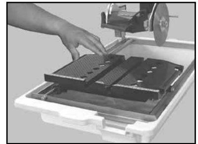
(F) Move Guide Bar and table until Square rests evenly across Blade
