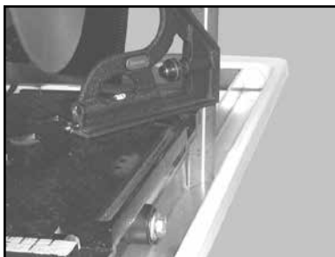
(H) Check that there is no gap between the Square and the wheel assembly side of frame
