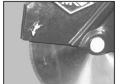
(F) Verify the Blade is seated on the Blade Shaft and direction of rotation is correct
